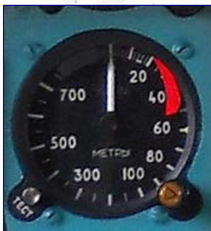
*Pointer Pressure altimeter in an airplane cockpit*
