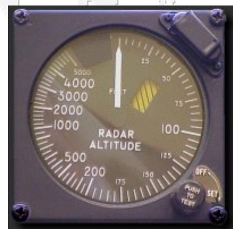
*Pointer Radar altimeter in an airplane cockpit*
