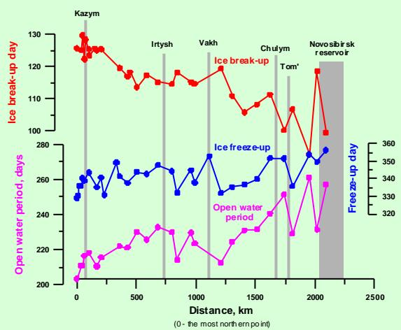
**Ice break-up and freeze-up day and duration of open water period along the main Ob' channel (Topex/Poseidon data)**
