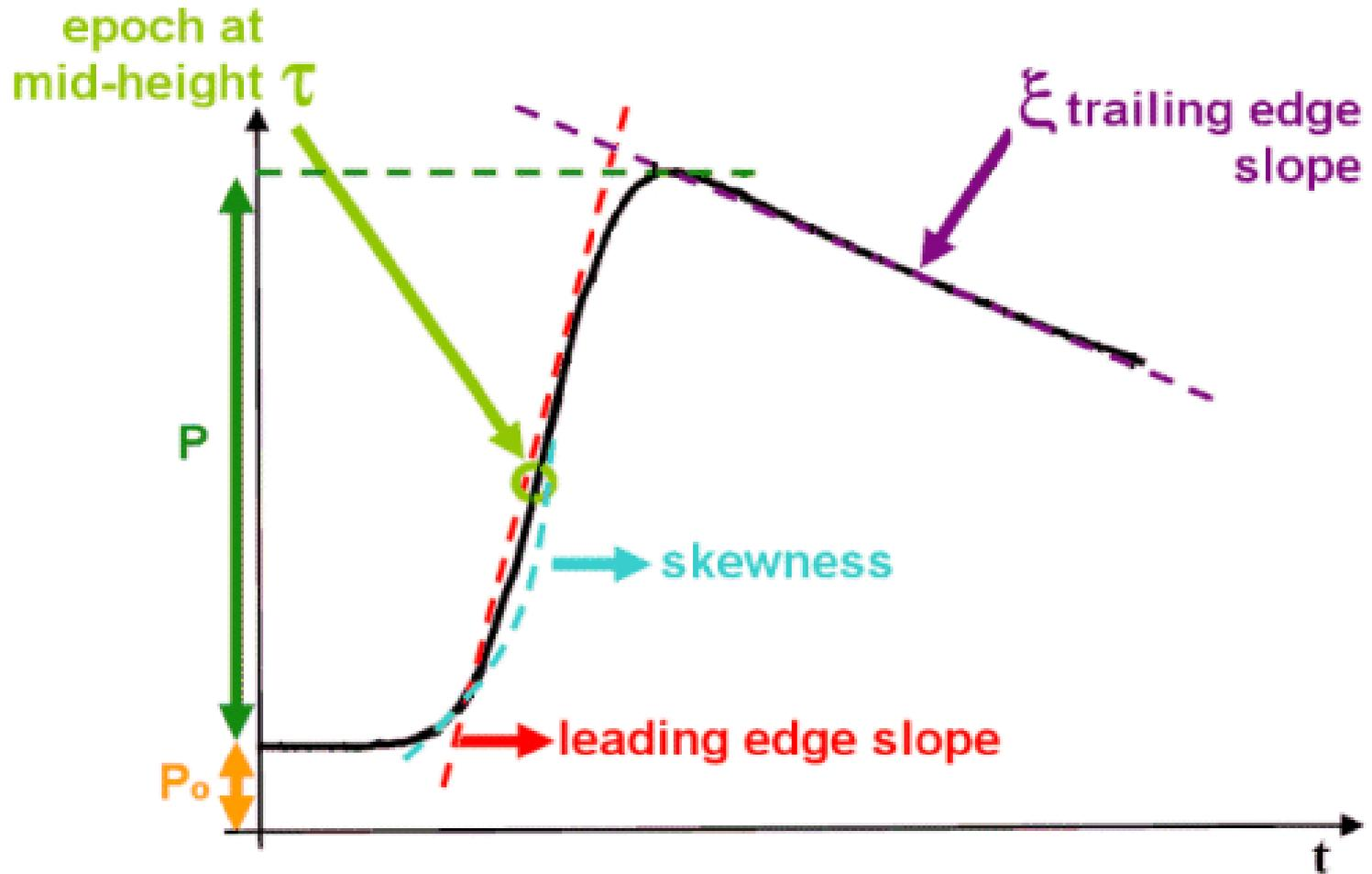
The waveform ( the shape of the reflected signal) represents the time evolution of the reflected power as the radar pulse hits the surface. In a definite time interval the signal is formed by the reflection from a definite footprint. This time interval is called a telemetric gate.
