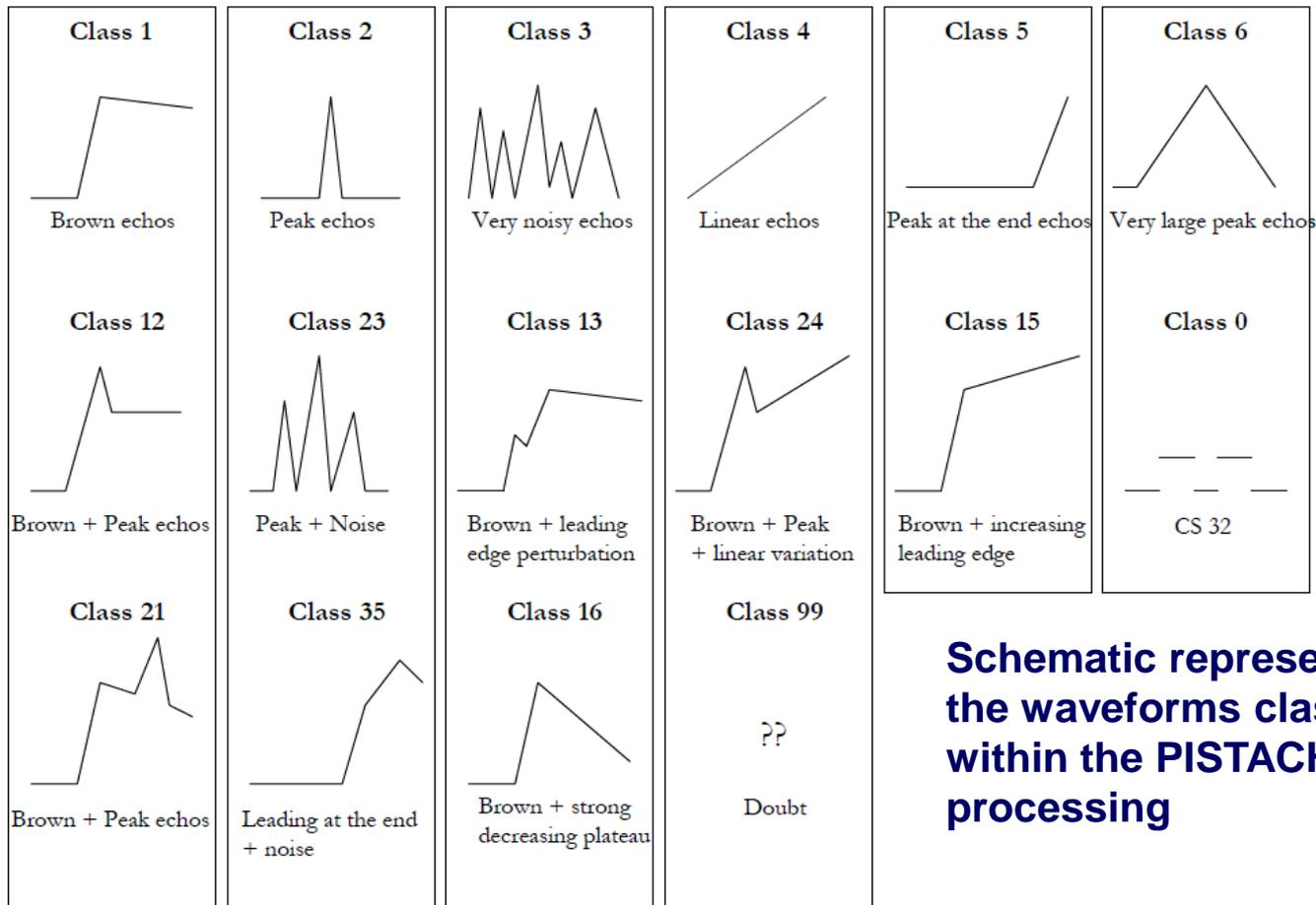
**Schematic representation of the waveforms classes within the PISTACH processing**
