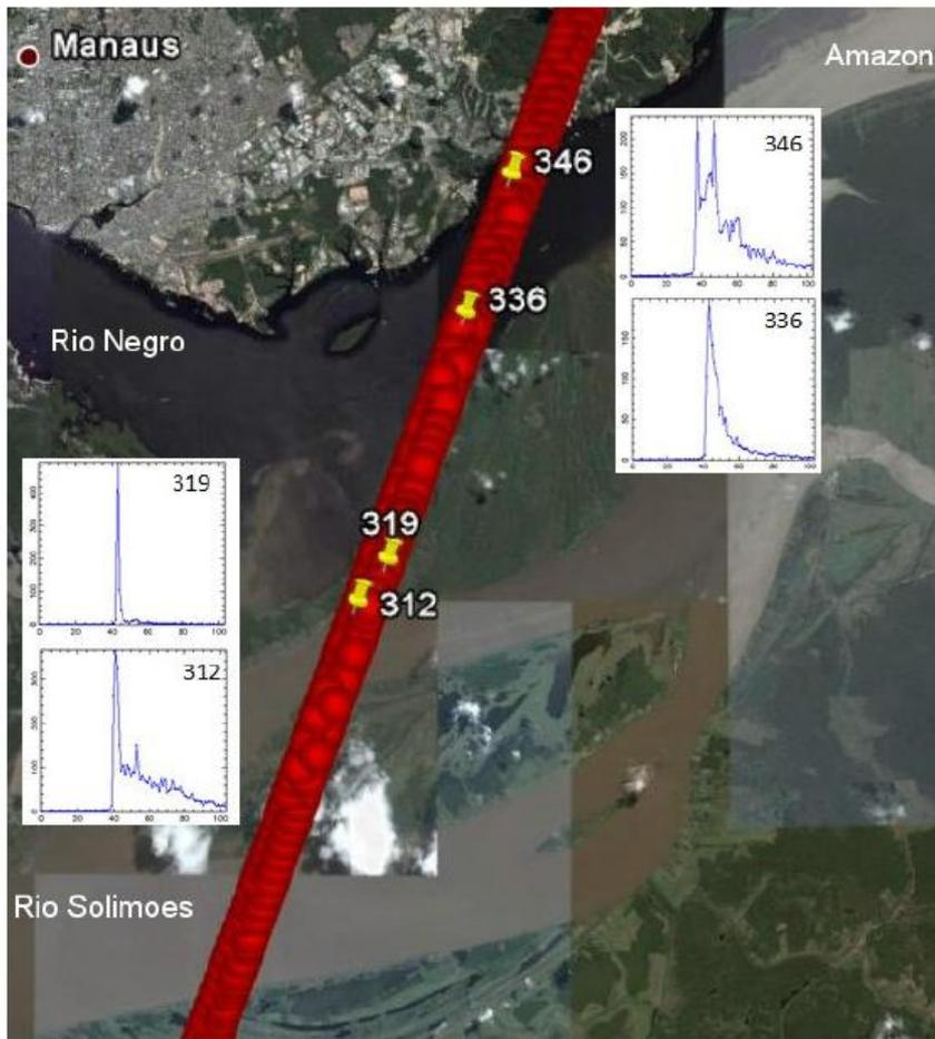
**Jason-2 waveforms on Amazon river : specular waveform (n°319) result of the return signal from very reflective surfaces like water bodies, multi-peaked waveforms result of heterogeneous targets in the footprint**
