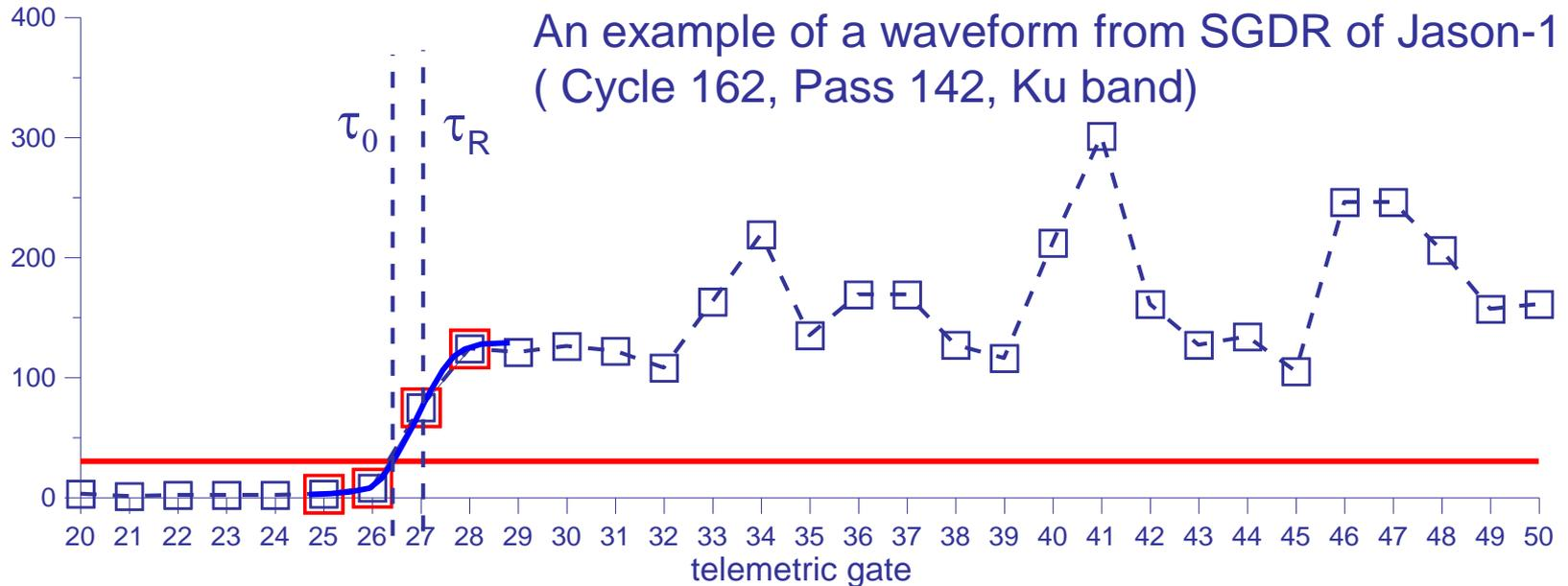
2. Improved threshold re-tracking algorithm. 4 points in the vicinity of the threshold are fitted by the error function
