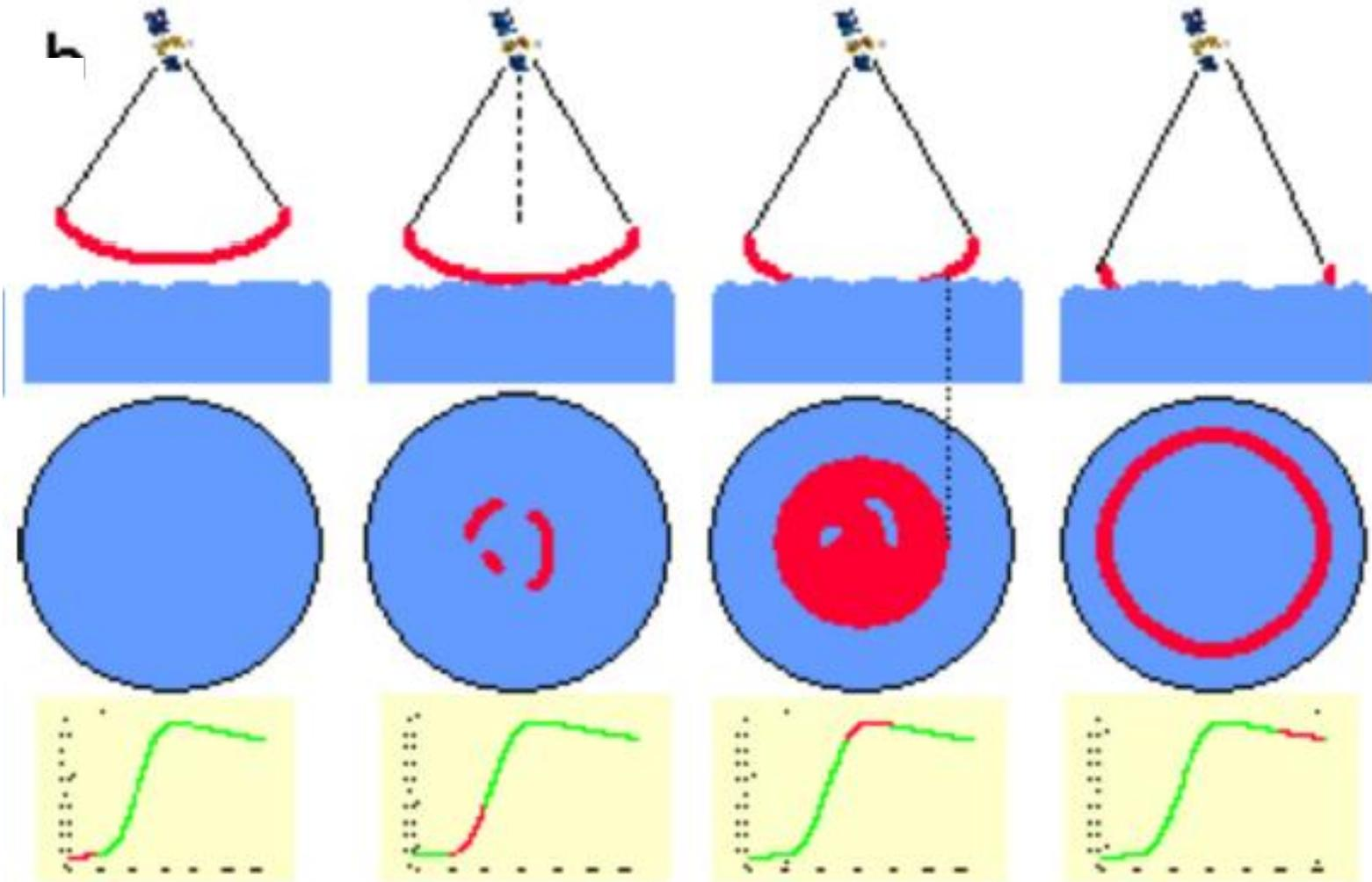
In sea swell or rough seas, the wave strikes the crest of one wave and then a series of other crests which cause the reflected wave's amplitude to increase more gradually. We can derive ocean wave height from the information in this reflected wave, since the slope of the curve representing its amplitude over time is proportional to wave height.
