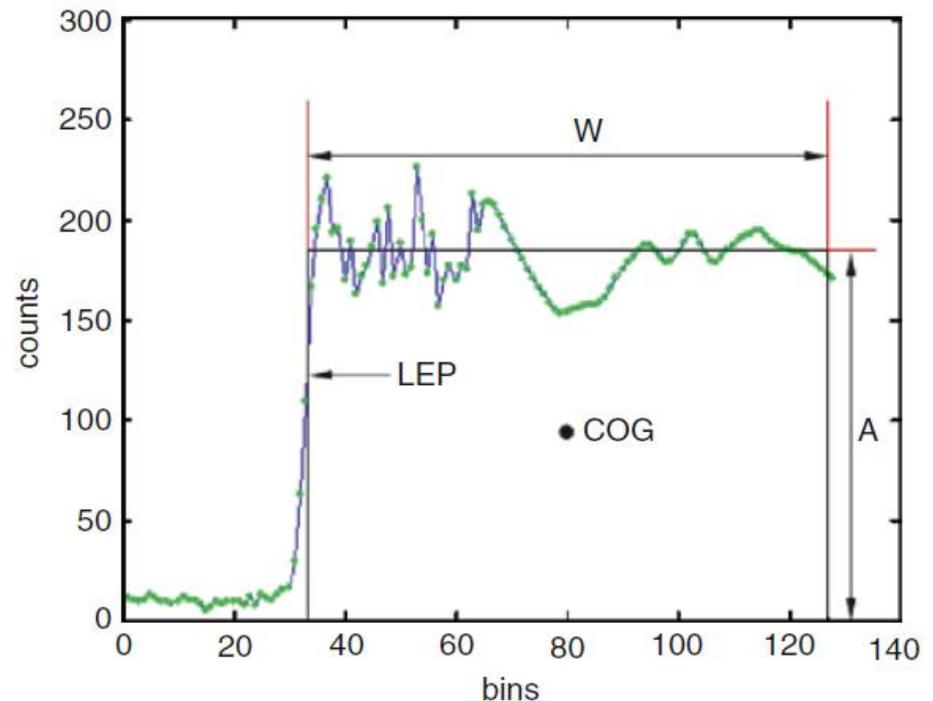
Schematic diagram of the OCOg method
