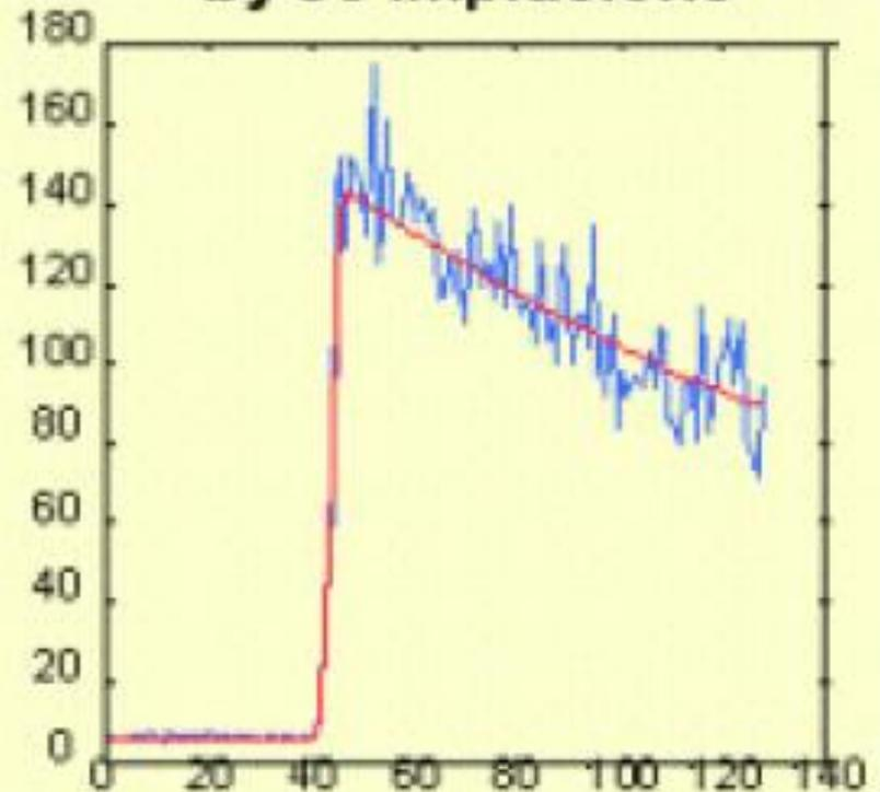
In practice, in sea swell or land, the illuminated surface is never flat. This effect is translated into a distortion and high frequency noise in the waveforms. To increase the signal/noise ratio, the individual echoes are averaged by 50 (ERS-1&2) or by 90 (Topex/Poseidon -Poseidon-1 altimeter- and Jason-1), making the elementary waveforms that will be transmitted to the ground.
