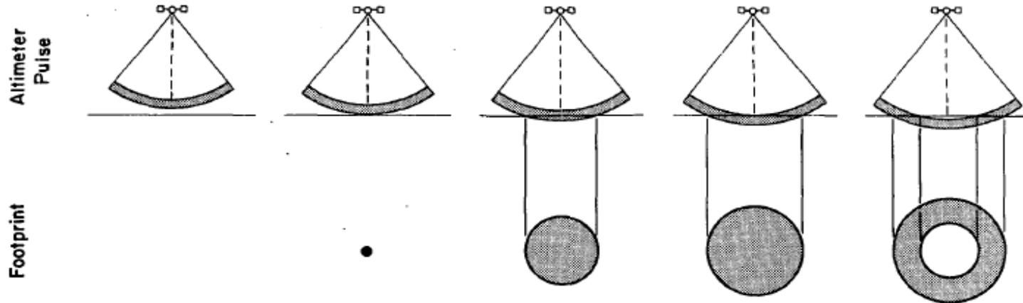
The radar altimeter receives the reflected wave (or echo), which varies in intensity over time. Where the sea surface is flat, the reflected wave's amplitude increases sharply from the moment the leading edge of the radar signal strikes the surface.
