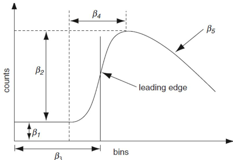
Schematic diagram of 5-parameter  $\beta$ -retracker waveform
