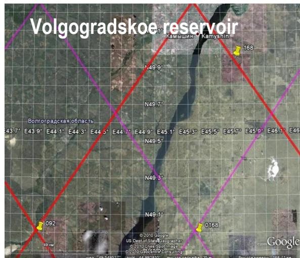
Main Volga River reservoirs with appropriate ground tracks of altimetry satellites Jason-1 and Jason-2: (a) Rybinsk Reservoir – 059 and 066 passes; (b) Gorky Reservoir – 142 and 0033 passes; (d) Kuibyshev Reservoir – 007, 142, 218 and 0218 passes; (e) Saratov Reservoir – 083 and 066 passes; (f) Volgograd Reservoir – 168 and 0168 passes
